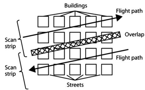
Fig. 3. Ideal urban grid pattern with standard flight pattern superimposed
